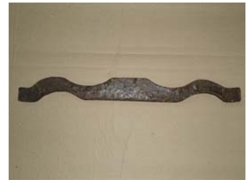
Yoke fabricated from composite material
