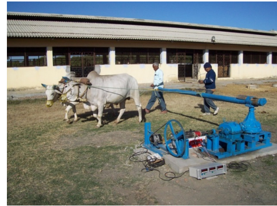
Rotary transmission system Suitable for charging two 12V Batteries- CAIE Bhopal Centre
