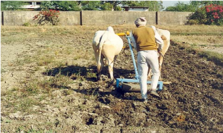
CIAE Bullock drawn blade harrow, Field capacity- 0.07 ha/h
