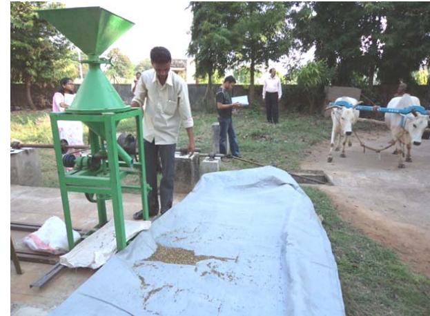
Adoption of Mini Dhal mill with rotary system- OUAT Bhubaneshwar
