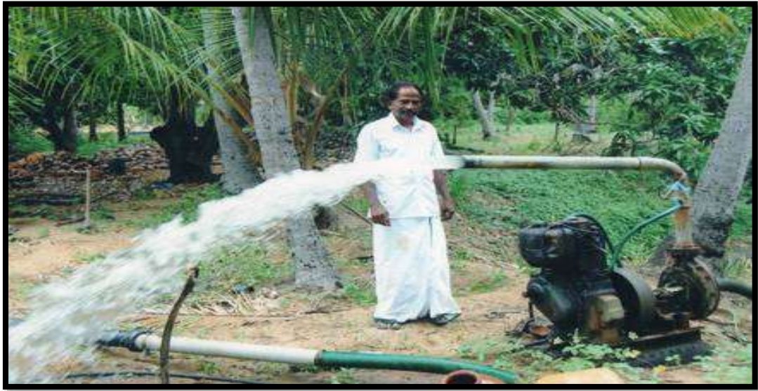
Fig. 8.6 Biodiesel engine for utilization of irrigation propose
