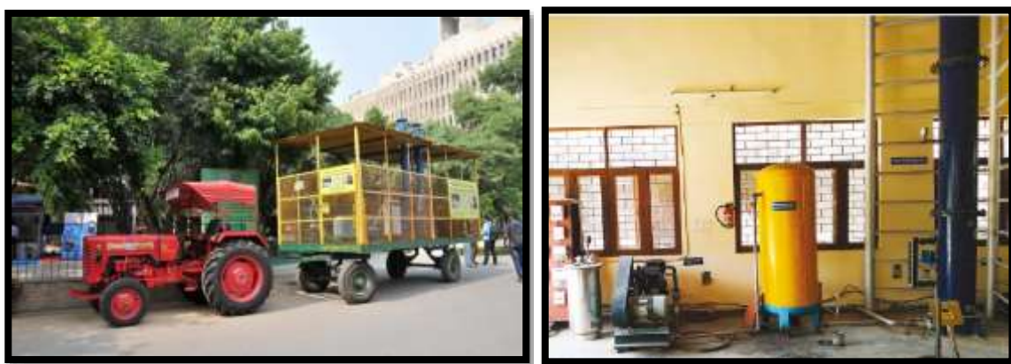
Fig. 3.2 Mobile & fix unit of Water scrubbing technology for biogas upgradation plant
