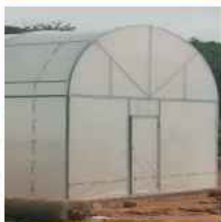
SOLAR TUNNEL GREENHOUSE DRYER COUPLED WITH BIOMASS BACKUP HEATER
