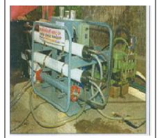
**Product/Process:** Reverse osmosis equipment. **Application/Use:** Desalination of brackish water (up to 10,000 ppm total dissolved solids) to get safe drinking water.
