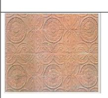
common clay is processed by wet grinding. Tiles can be fabricated in different shapes, sizes and designs. These are fired in an improved up draught kiln at 1000°C-1100°C. Different transparent/color glazes can also be provided subsequently.
