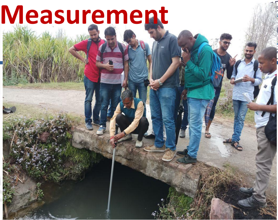
Flow measurement using hand held velocity metre
