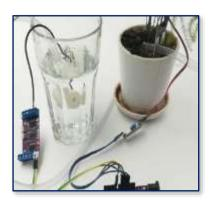
irrigates the plant. After supplying sufficient water, the soil get retains the moisture hence automatically stopping the pump.
