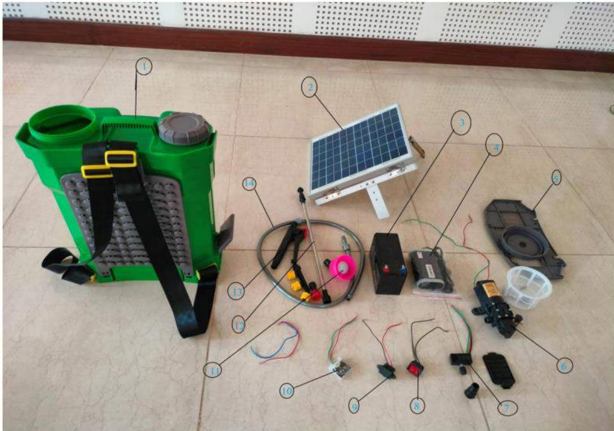
Fig 2: Components of solar powered fertilizer sprayer
