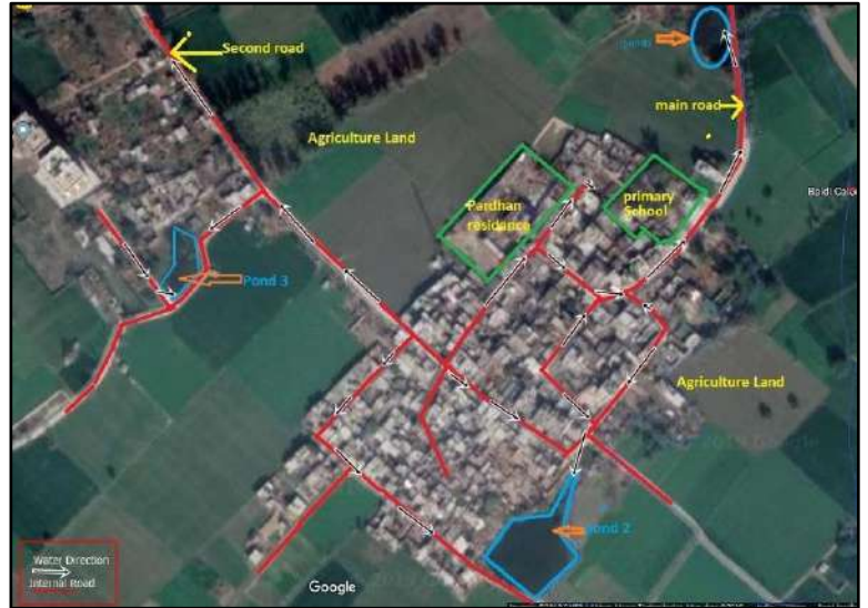
Existing drainage pattern in the village identified through ground survey
