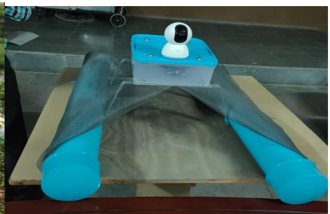
Fig.8 Solar Aqua Skimmer for cleaning the wastages in the lake
